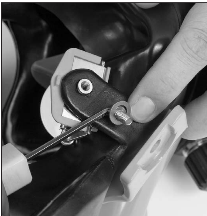
Insert the screw through the mask frame.
