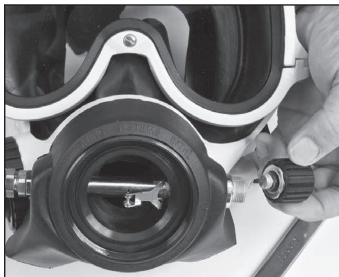
Unscrew the adjustment knob assembly from the regulator.
