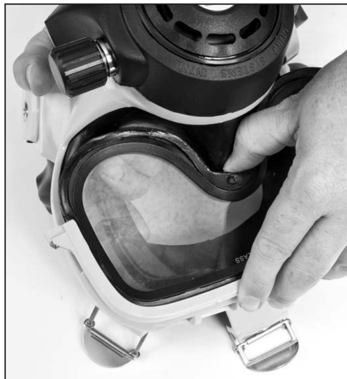
Adjust the seal around the bottom of the lens.
