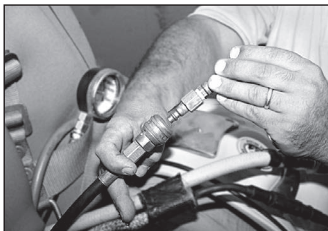
The use of a quick-disconnect fitting makes using the mask much easier for surface-supplied diving.
