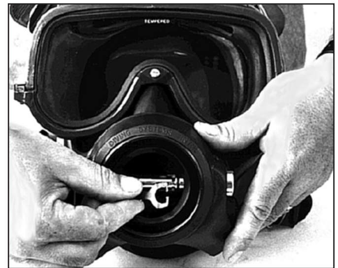
Remove the roller lever arm.
