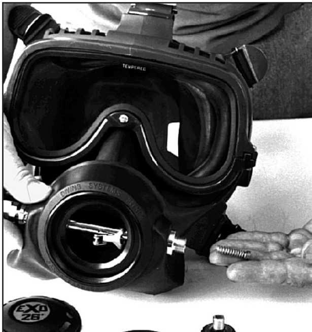
Remove the spring and spacers. the washer and diaphragm.
