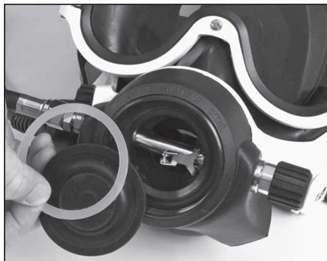
Remove the diaphragm and washer.
