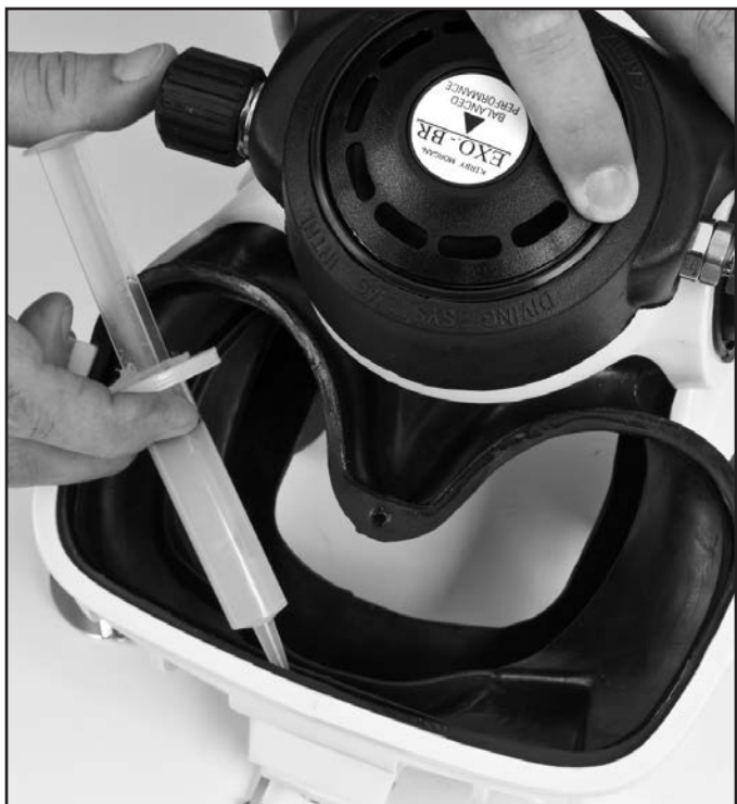
Apply silicone grease to the mask seal.
