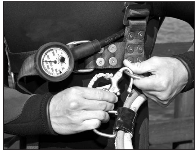
The bail-out system must have a submersible pressure gauge for the diver to monitor the gas supply.
