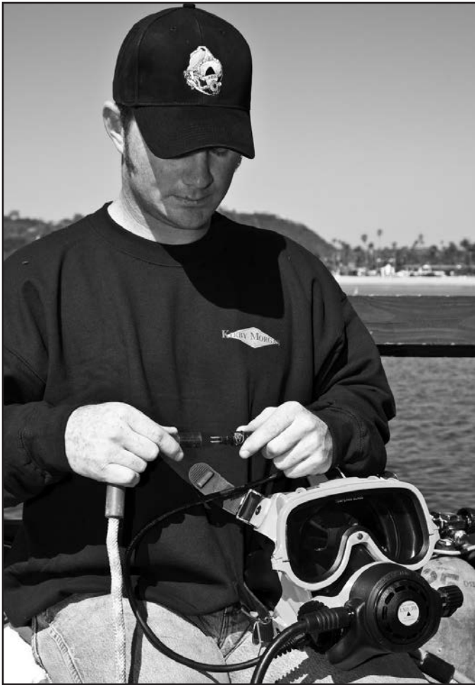
Connect the waterproof connectors without twisting them.
