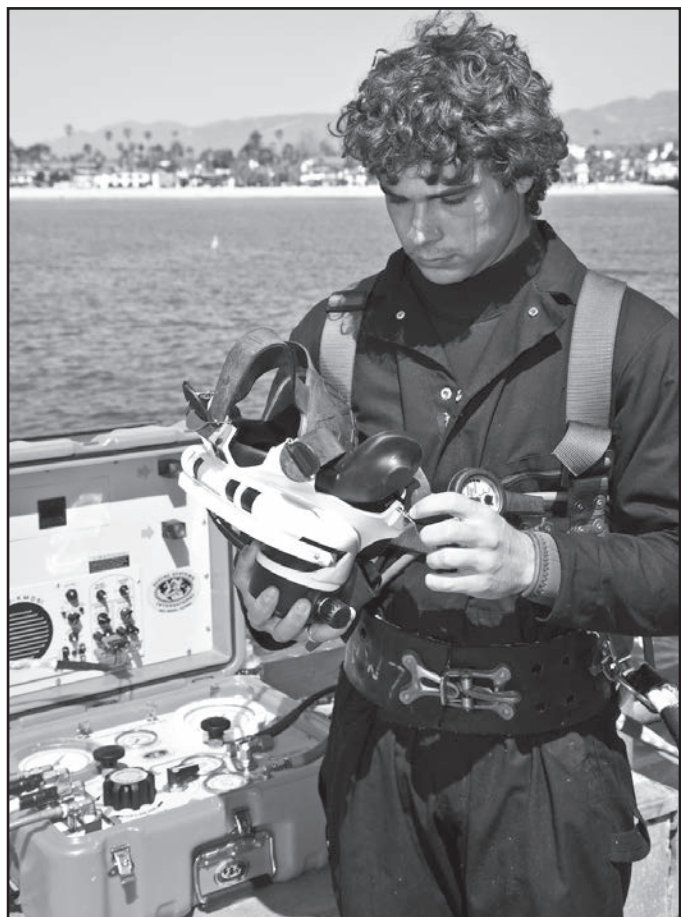
The EXO-BR works well in the surface-supplied mode.
