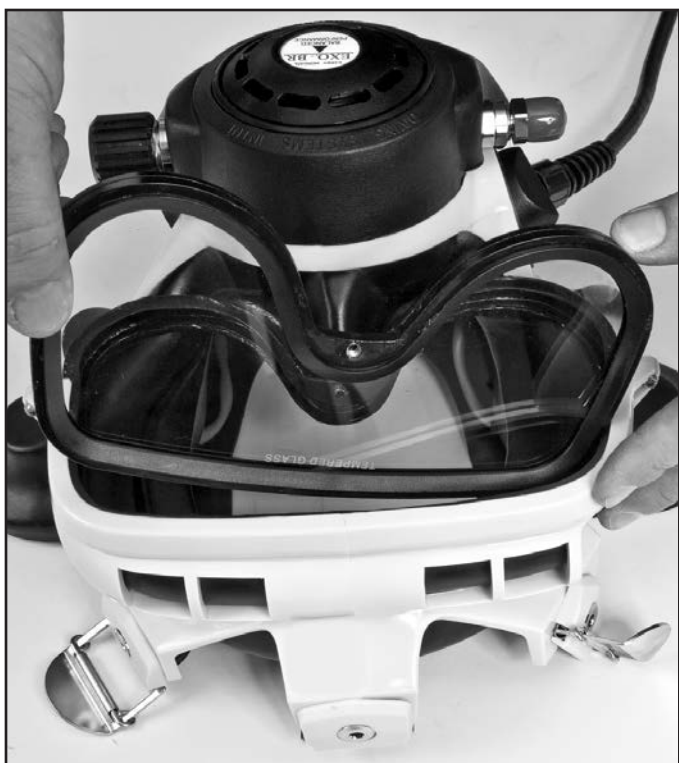
Install the right side of the lens rim into the channel of the rubber on the mask seal.
