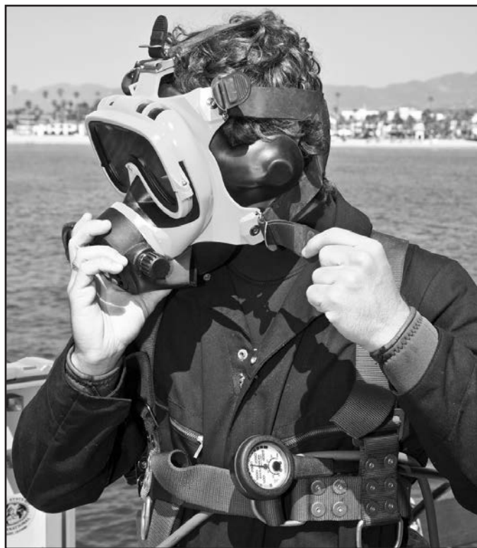
Tighten the lower spider legs first.
