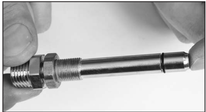
Inspect the nipple tube seating surface for dings, nicks, and wear. You should be able to feel any irregularities with your fingernail.
