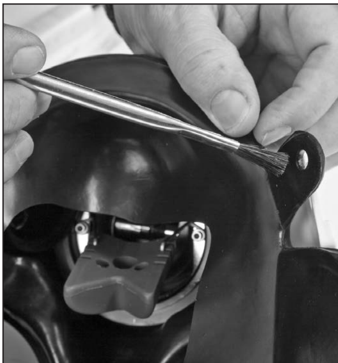
Lightly lubricate the screw hole on the spider tab.
