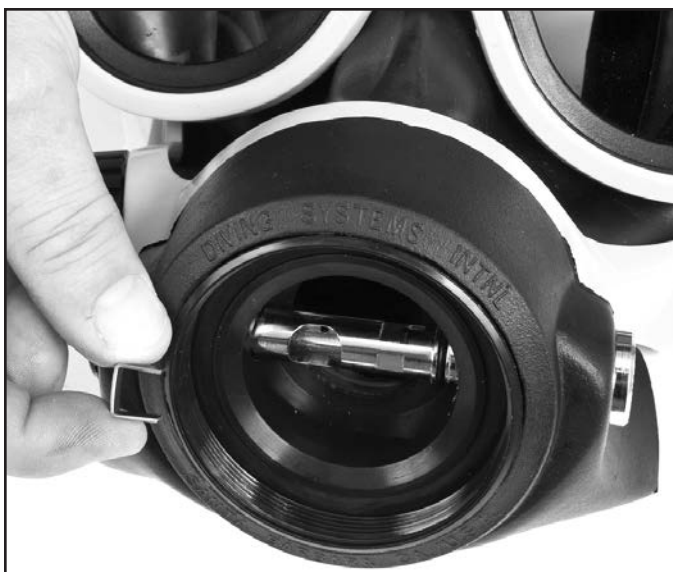
The horseshoe is critical to the proper function of the regulator.
