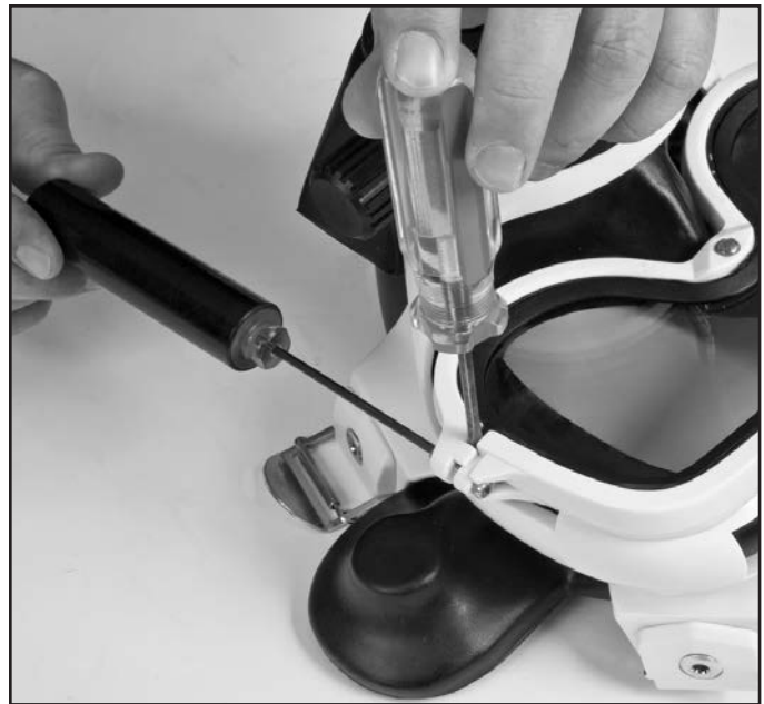
Use a flat blade screwdriver to keep the mask seal from pinching as the lens clamp is tightened.
