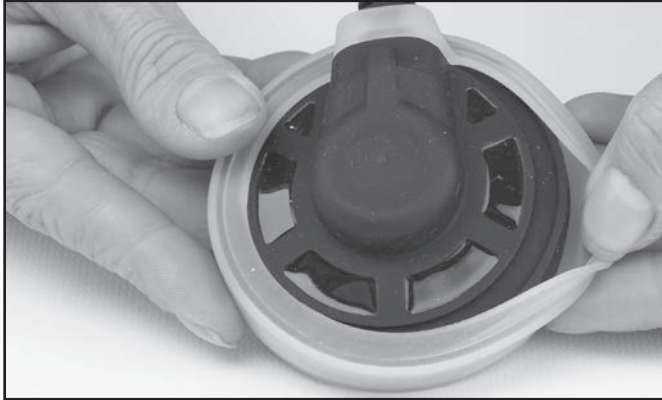
Remove the outer earphone covers and allow all the parts to dry.
